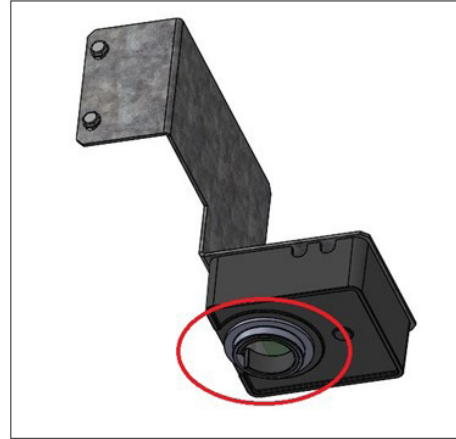
Fig. 2. Ice level sensor lens location.
