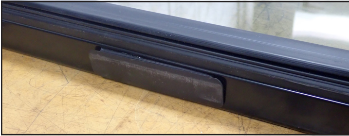
Fig. 11. Wire cover located in the hinge-side of the door in the center.
