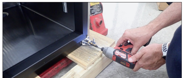
Fig. 7. Install the bottom hinge on the opposite side of the door opening.
