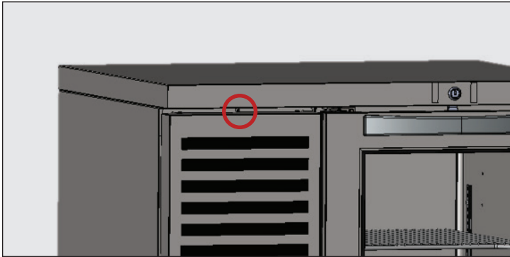
Fig. 1. Louver grill screw location.
