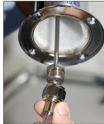
Fig. 3. Attach the beer line connector to the draft arm.
