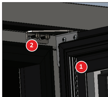
Fig. 10. Install the top hinge and the door.
