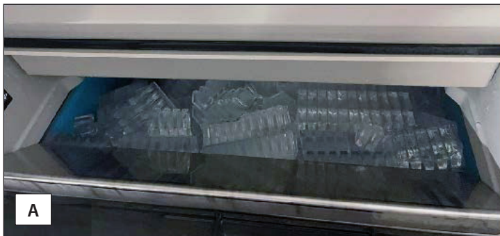
Fig. 5. Ice bins with (A) and without (B) a drop-zone deflector.
