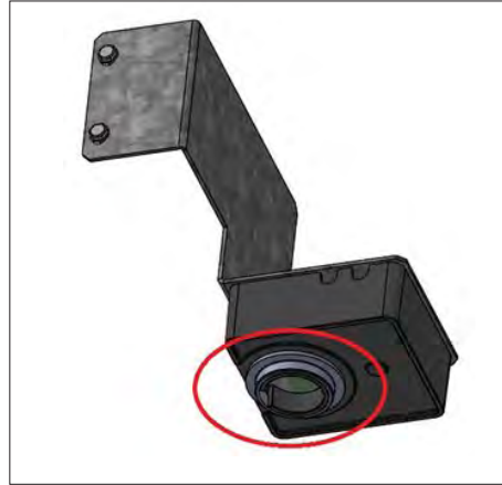
Fig. 2. Ice level sensor lens location.
