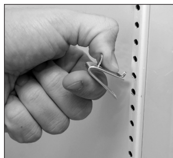
Fig. 1. Installing top tab of shelf clip.
