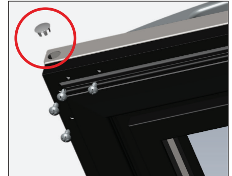
Fig. 6. Remove the door plugs and remaining screws.
