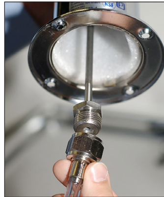
Fig. 3. Attach the beer line connector to the draft arm.
