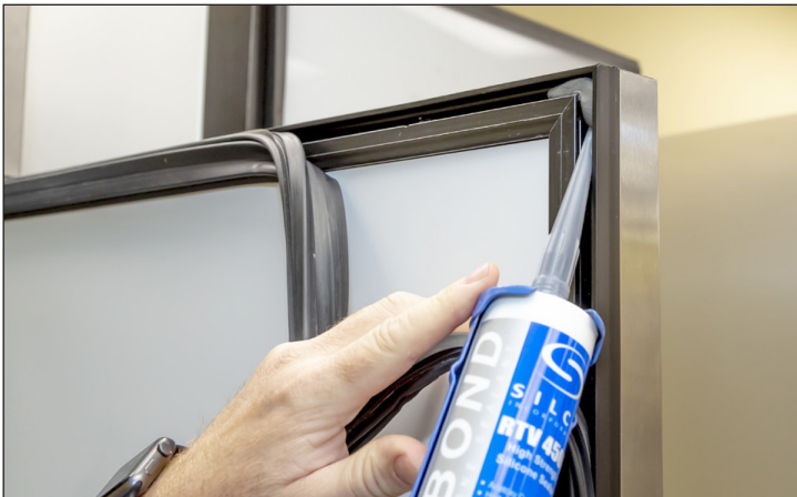
Fig. 3. Apply silicone to each corner of the gasket channel.
